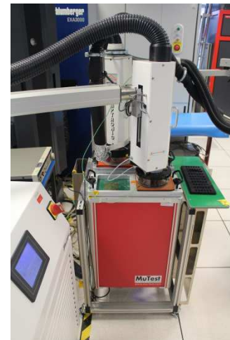
Figure 1: Mutest ATE with ThermoStream to characterize components
