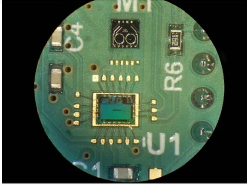
Figure 3: PCB with ASIC and MEMS
