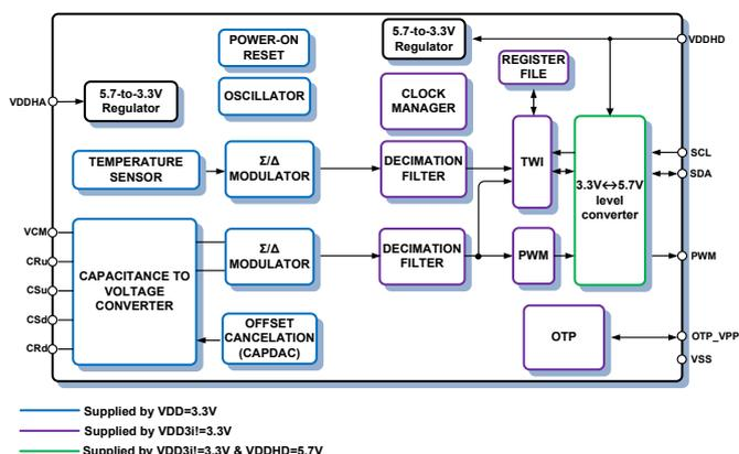
Figure 1: Functional block diagram of ASIC
