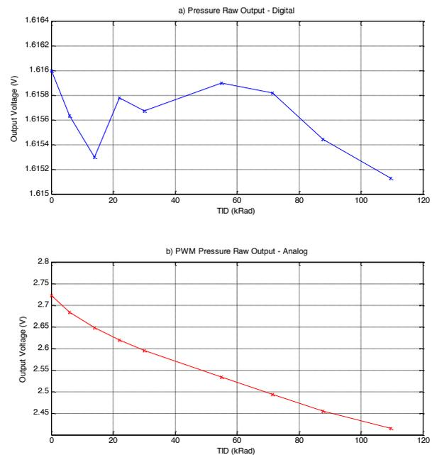
Figure 5: a) Pressure raw digital output b) PWM pressure output vs. TID dose
