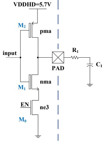
Figure 6: Output stage of 3.3V-to-5.7V level converter and RC filter
