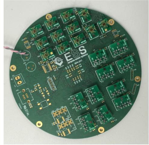
Figure 4: PCB with mounted DUTs for TID
