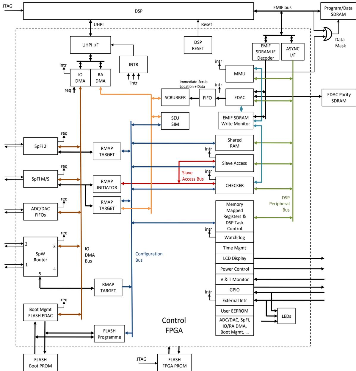
Figure 5: Block Diagram of HPPDSP FPGA Architecture
