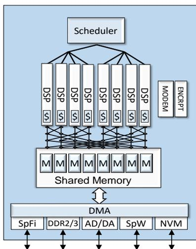
Figure 4: RC64 Architecture (only 8 DSP processors are shown)
