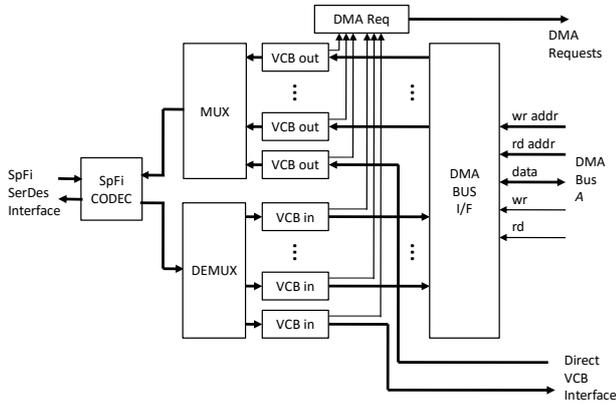
Figure 3: SpaceFibre Interface Block Diagram
