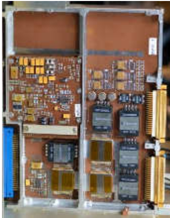
Figure 10: RTU board with the plugin module @ center left
