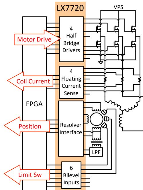
Figure 1: Block diagram of Motor Control System
