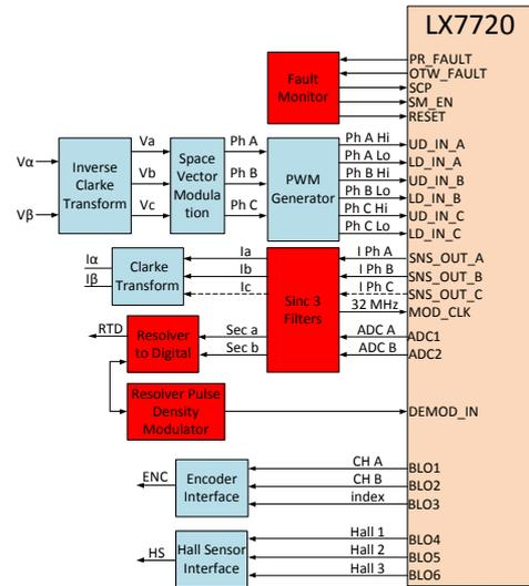
Figure 7: PMSM IP blocks using LX7720
