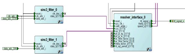
Figure 9: Development of Resolver to digital IP Blocks
