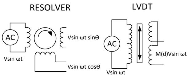
Figure 4: Resolver and LVDT
