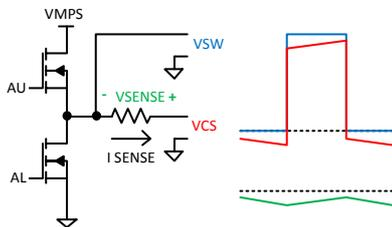
Figure 3: In-line current sense on switch node
