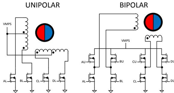
Figure 2: Two phase stepper motor configurations
