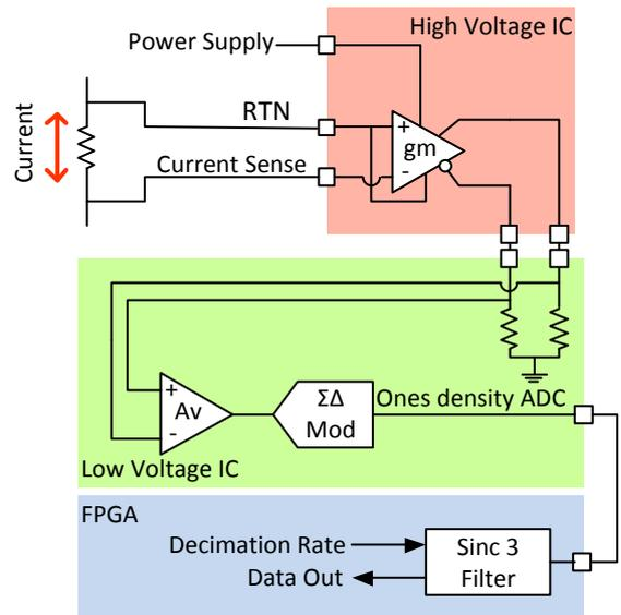
Figure 5: Floating current sense design
