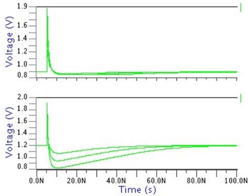
Figure 2: Single event simulation of a buffer connected two stage OTA at the high impedance node of the input stage (upper curve). The lower curve is the output of the OTA.
