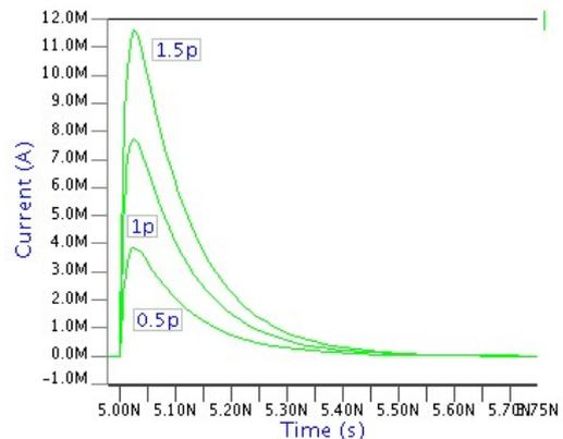
Figure 1: Current pulse for single event simulation
