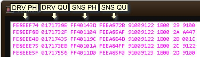
Figure 11 Data frames from DPC to OBC on the UART port (115200 bauds).
