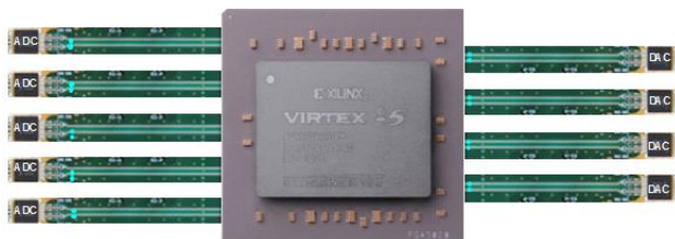
Figure 5: Serial ADCs/DACs connected to a space-grade FPGA
