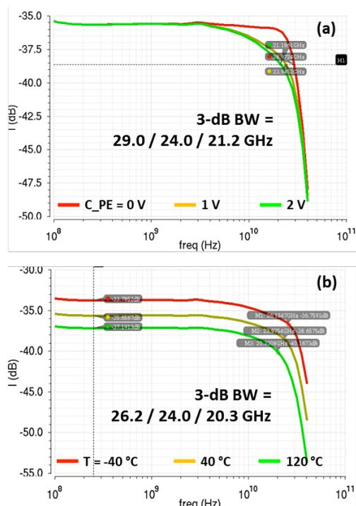
Figure 2: Post-layout simulated frequency responses of VCSEL driver at different (a) pre-emphasis levels and (b) operating temperatures.
