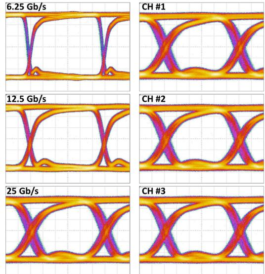
Figure 11: Measured eye diagrams of Gen-1 TIA.
