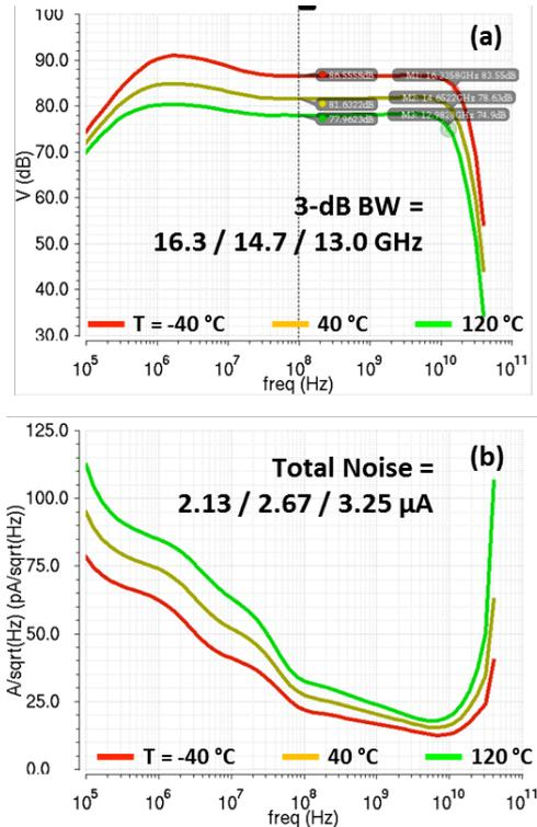
Figure 5: Post-layout simulated (a) transimpedance gain and (b) input-referred noise current density responses of TIA at different operating temperatures.
