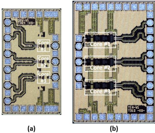
Figure 9: Chip photos of Gen-1 VCSEL driver and TIA.
