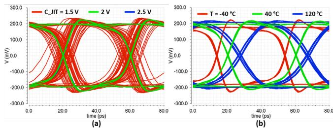
Figure 6: Post-layout simulated eye diagrams of VCSEL driver at different (a) jitter optimizations and (b) operating temperatures.
