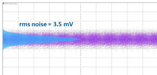
Figure 12: Measured output noise voltage of Gen-1 TIA.
