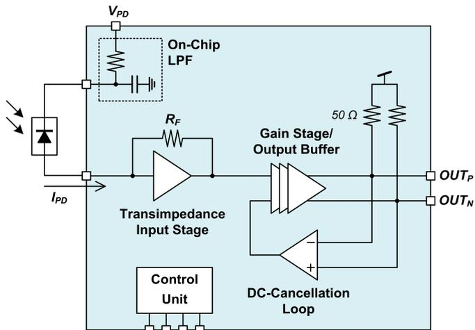
Figure 4: Schematic of TIA core.
