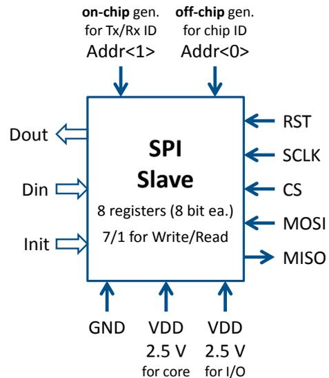
Figure 8: Block diagram of SPI.
