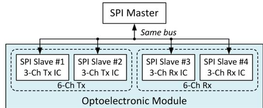
Figure 7: Serial communication interface configuration for 6-channel optoelectronic module.
