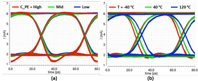
Figure 3: Post-layout simulated eye diagrams of VCSEL driver at different (a) pre-emphasis levels and (b) operating temperatures.
