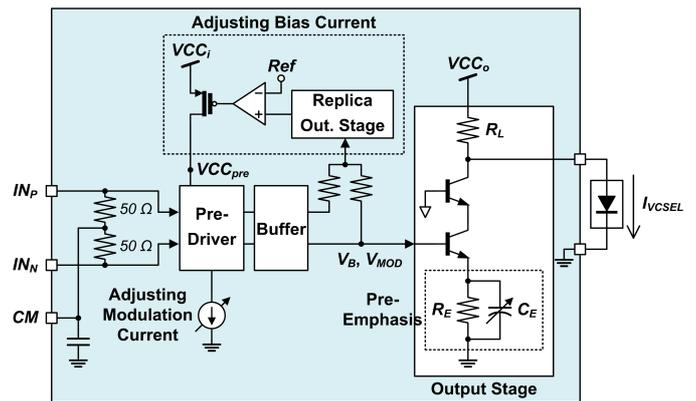
Figure 1: Schematic of VCSEL driver core.
