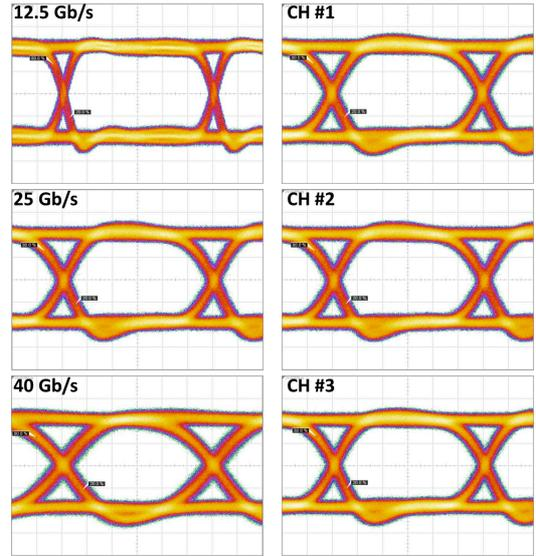
Figure 10: Measured eye diagrams of Gen-1 VCSEL driver.
