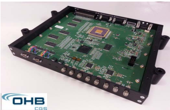
Figure 5: DSP board developed by OHB CGS with Texas Instrument TMS320C6727 DSPs.
