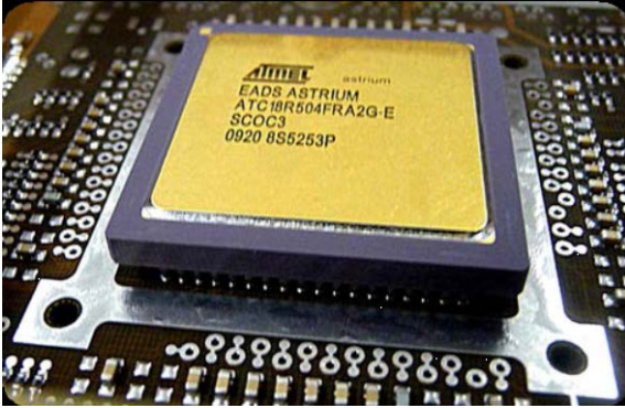
Figure 4: HiP-CBC SmartIO prototype is implemented with a SCOC3ASIC.
