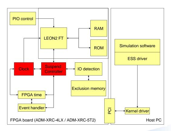
Key function Suspend Controller will suspend Leon while simulating I/O
