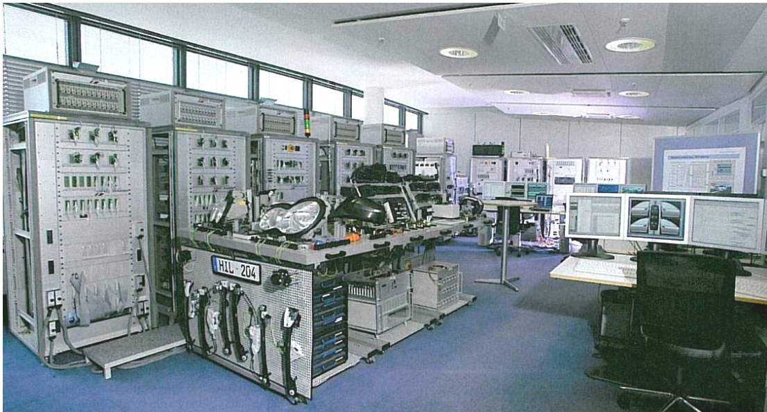
Fig. 1: Virtual vehicle HIL system for testing a mid-range vehicle ([1])
