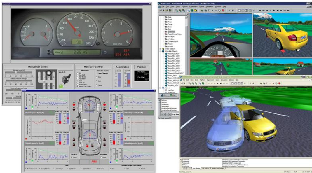
Fig. 4: ControlDesk for interactive operation of the HIL systems and MotionDesk for 3-D visualization [5]
