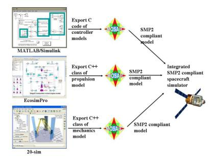
Fig. 7. Example use case scheme of MOSAIC 9, transferring domain specific models (e.g. controller, propulsion and mechanics) from different model development environments to SMP2.
