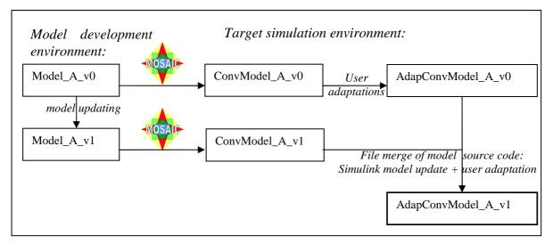
Fig. 4. Process illustration of the merging of simulation model versions.
