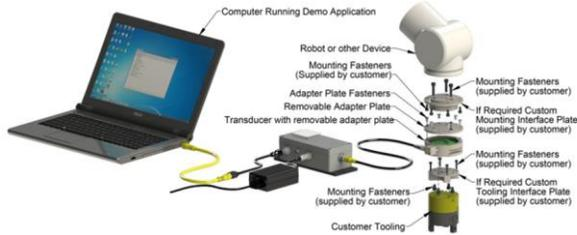
Figure 6: Load cell
