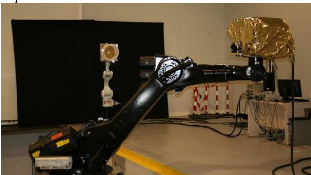
Figure 4: Servicing docking scenario dynamic test set-up during HARVD activity
