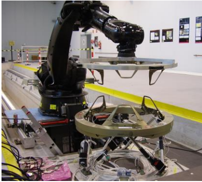
Figure 3: Support of platform-art to IBDM EDU contact/docking tests
