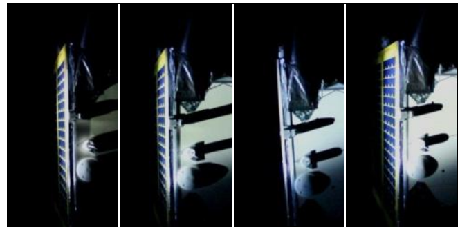
Figure 6: Sequence of short-range PRISMA-TANGO S/C mockup lab images with different illumination directions
