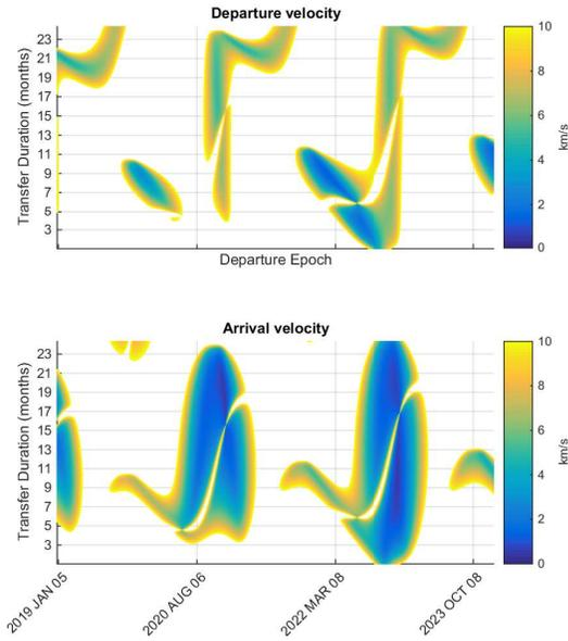
**Fig. 1.** Pork-chop plot associated to AIM interplanetary transfer through bi-impulsive maneuver.
