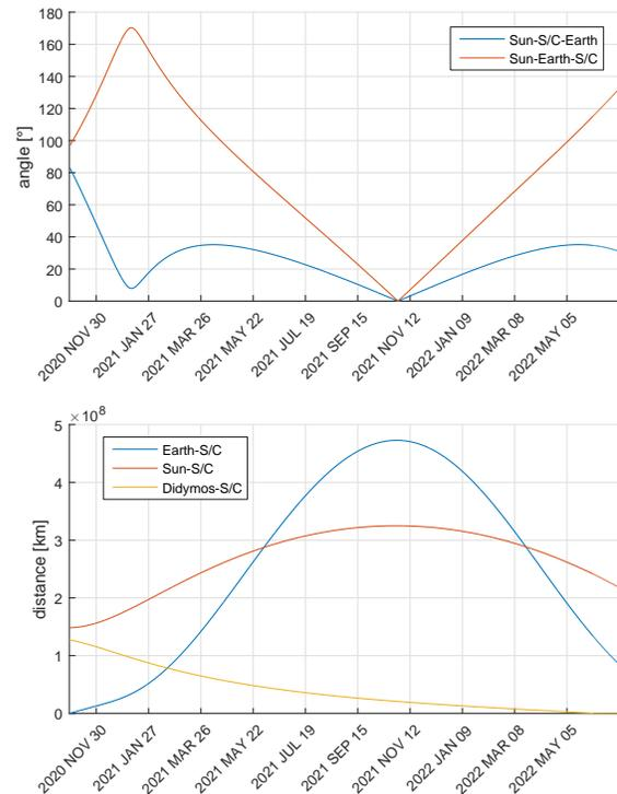
**Fig. 3.** Sun-S/C-Earth and Sun-Earth-S/C angles, with Earth, Sun and Didymos distances from the spacecraft during interplanetary transfer.
