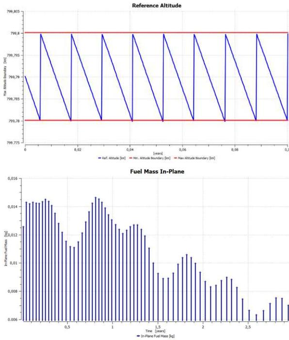
Figure 10. Altitude Control (above) and Firing Fuel Mass History (below)
