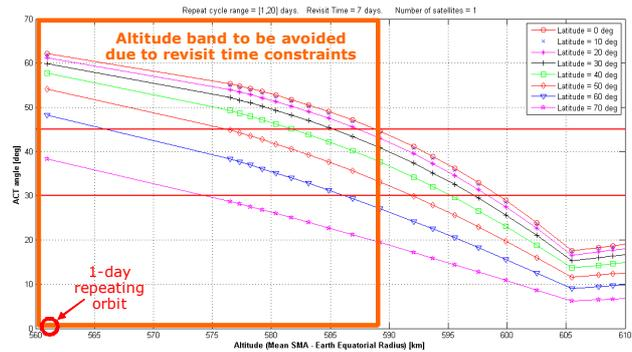
Figure 19. Required Across-Track Angle for Global Coverage
