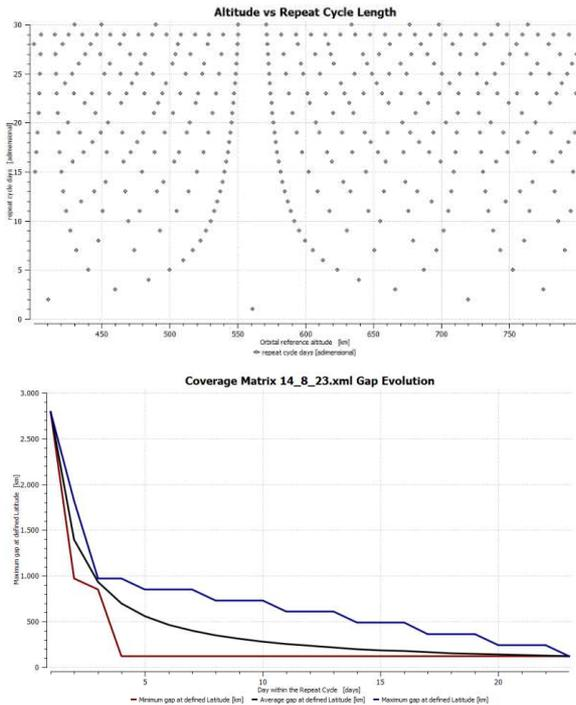
Figure 14. Altitude vs. Repeat Cycle Map (above) and Gap Evolution Graph (below)
