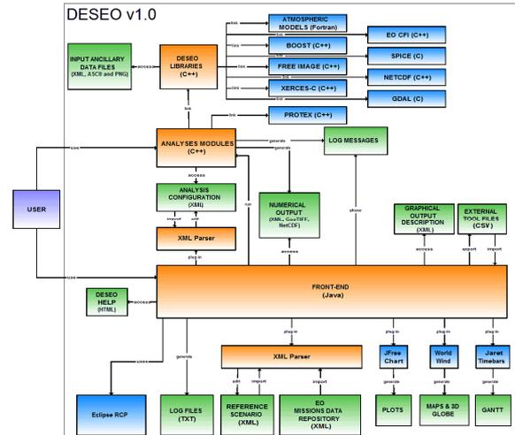
Figure 1. High-Level System Decomposition
