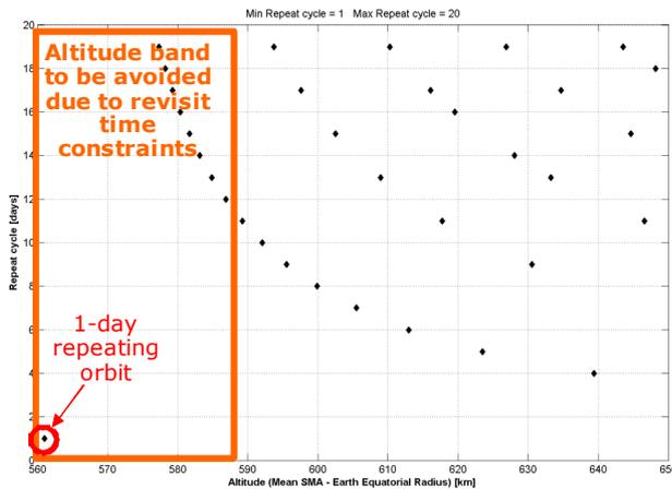
Figure 18. SSOs Repeating Orbits Plot
