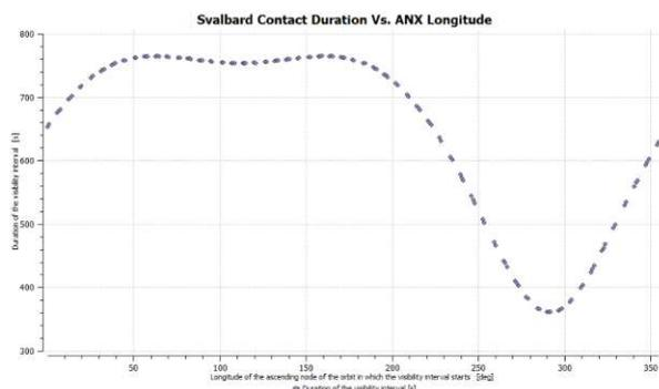
Figure 7. GS Contact Duration vs. Ascending Node Crossing Longitude
