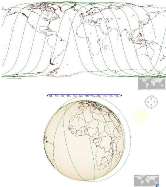
Figure 2. Propagated Orbit: Map Projection (above) and 3D View (below)
