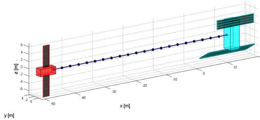
**Figure 4. Multibody model used for simulations (20 nodes tether discretization)**
