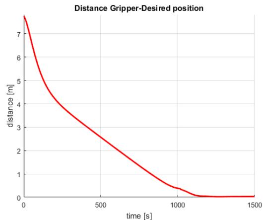
Figure 18. Distance between grappling point and gripper location
