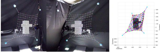
**Figure 12. Net trajectory 3D reconstruction of parabolic flight experiment**
