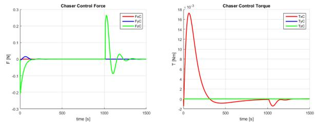
Figure 16. Chaser control forces and torques (chaser body frame)
