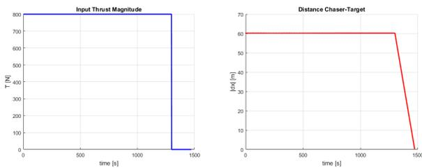
Figure 5. Input step profile and relative distance evolution
