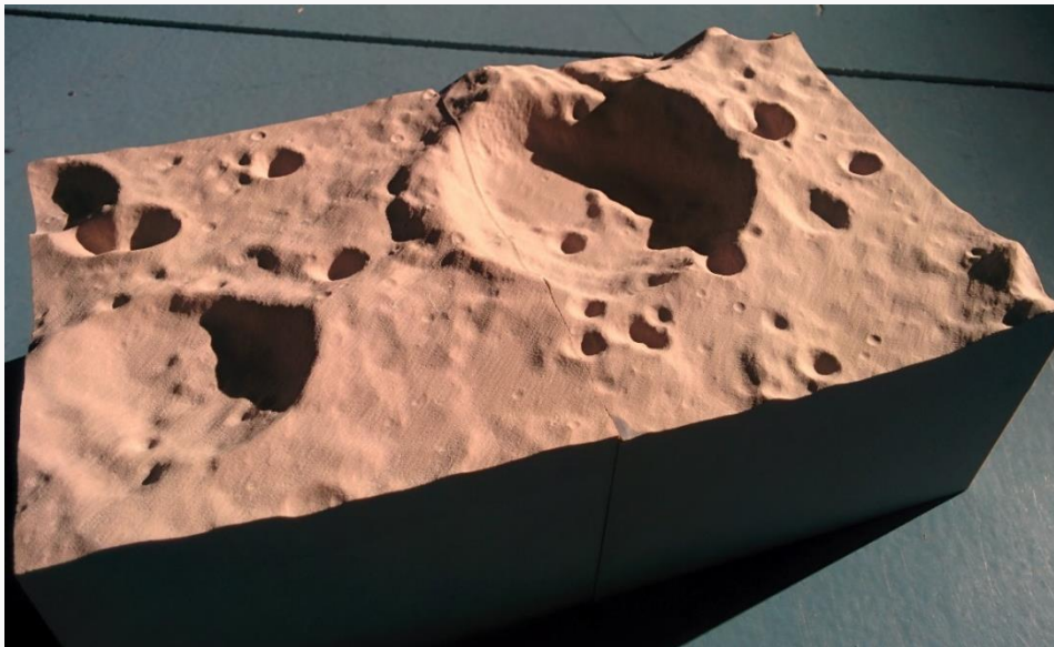
Lunar surface sample milled with a 5 mm spherical cutter and a milling step of 0.2 mm
