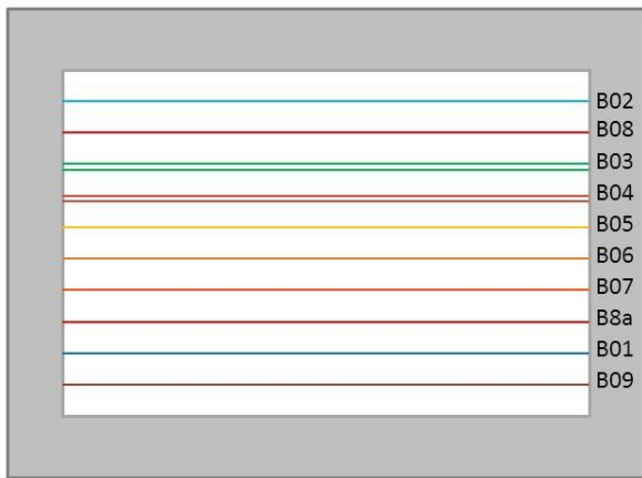
Fig. 5. Schematic view of one VNIR detector
