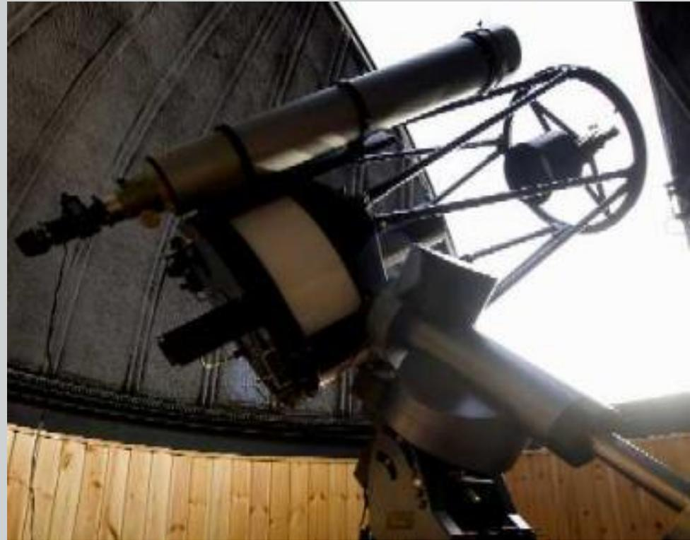
A FLI CCD camera, model ProLine PL09000 3056 x 3056 pixel Front-Illuminated with sensor ON Semi KAF-09000 - pixel size:12  $\mu\text{m}$  ,USB 2.0 is connected to the [RCOS](#) telescope at direct focus
