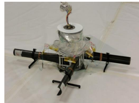
Packaged Inflatable; Combined Inflatable and Deployable Boom Mechanism
