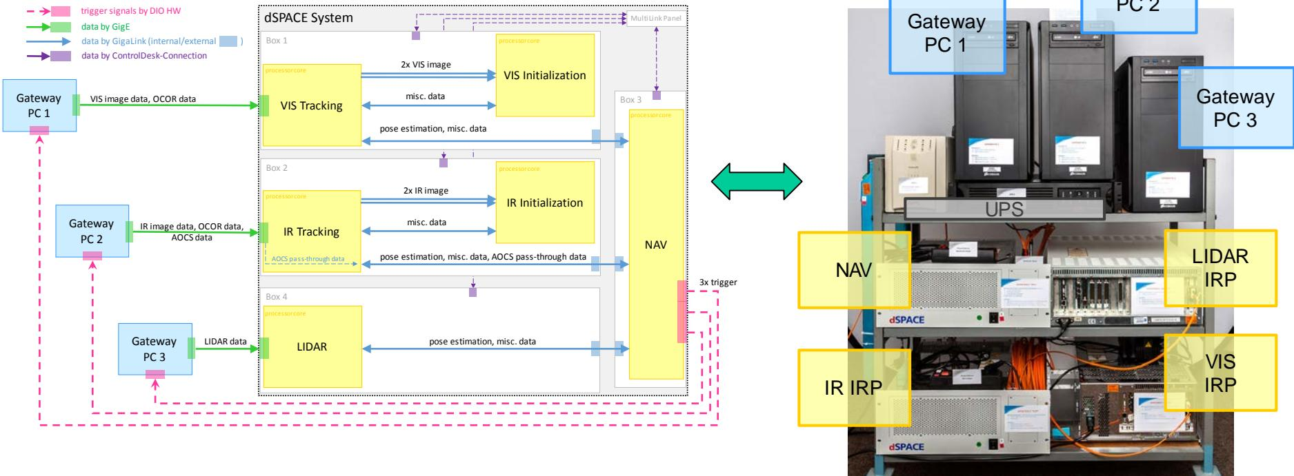
→ PIL Tests currently running (prelim. result: performance comparable to MIL tests)
