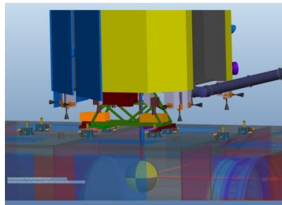
Lowering to the 4th row while keeping contact with the 3rd row (robotic arm + cameras + guiding elements)
