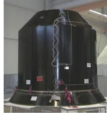
SYLDA Ariane 5 Multiple Payload Dispenser
