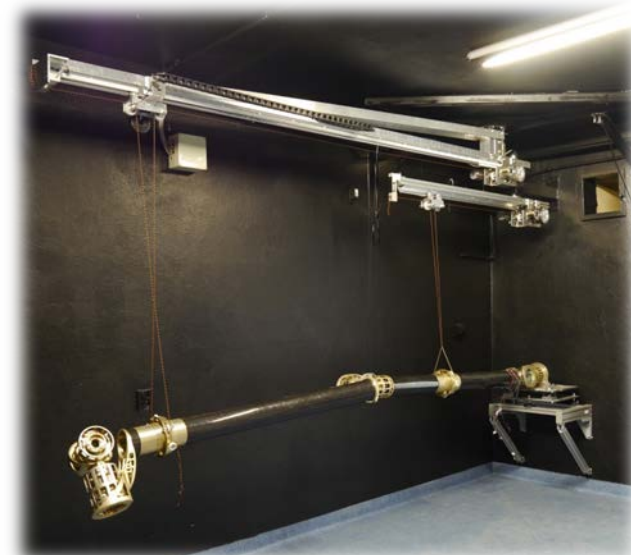
Weight-reducing suspension system at CBK PAN.
