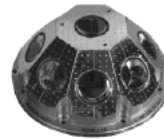
Retroreflector array of Envisat. Courtesy of ESA
