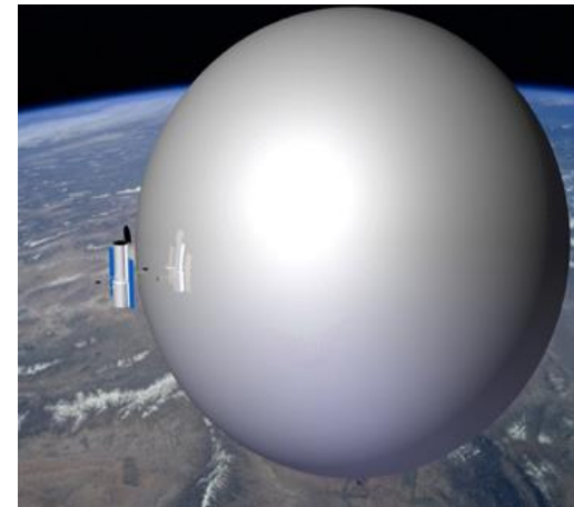
Example: Gossamer Orbit Lowering Device by Global Aerospace Corp
