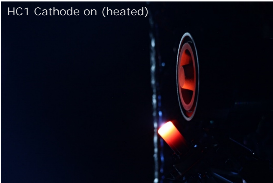
HT100 + HC1: Thruster Unit Operating at nominal power (175W)
