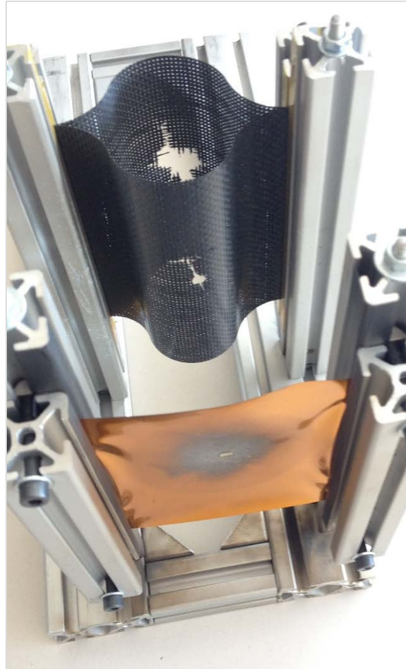
Boom impact tests, source TUM
