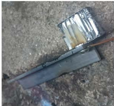
336°C discoloration evident; conduction slow
