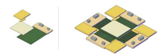
Possible simple drawing of two layers (SiL + SFL) and SiPM and of a complete 8 layer apparatus (4+4)
