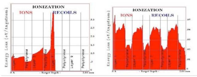
Energy released in the device by a minimum energy particle (left) and minimum ionizing particle (right), Z = 1
