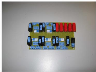
Breadboard and laboratory DM models constructed
