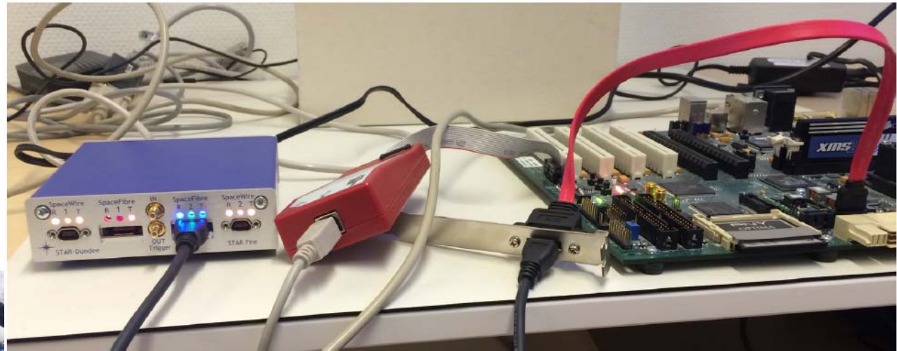
Interoperability test between Gaisler's SpaceFibre IP (on Virtex-5) and STAR-Dundee's STAR-Fire unit
