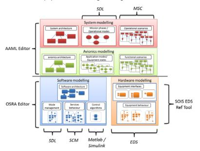
The toolset includes additional capabilities such as state machine simulation, code generation, and documentation generation, representing a complete framework for the development of space systems.
