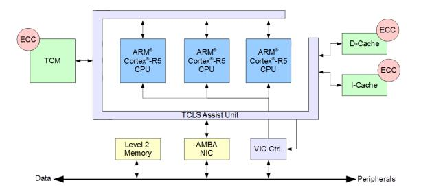
• **3 ARM CPUs** (e.g., Cortex-R5) to be implemented using **commercial process technology**
