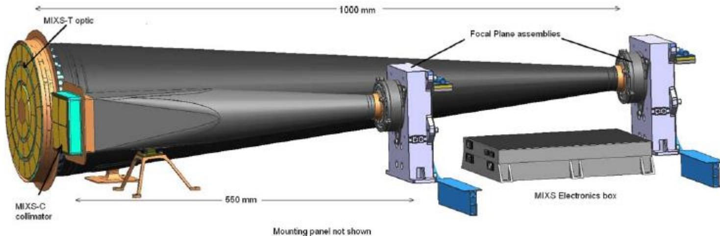
Fig. 1. A Schematic illustration of MIXS showing the adjacent MIXS-T and MIXS-C channels.
