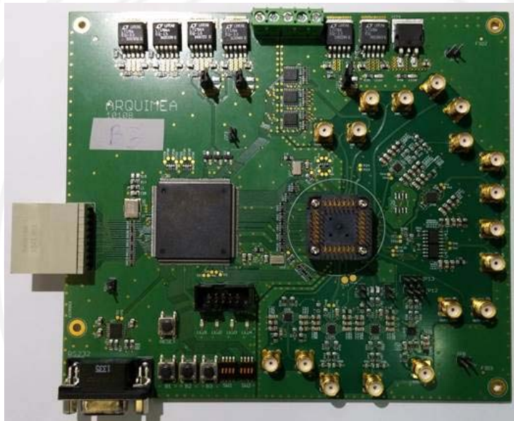
ARQ-CVA001 functional test board and setup at ARQ facilities
