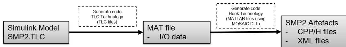
Fig. 6 STF/MOSAIC code generation workflow from Simulink
