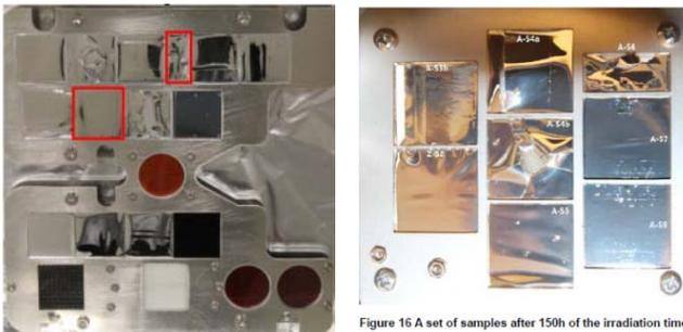
Figure 16 A set of samples after 150h of the irradiation time.
