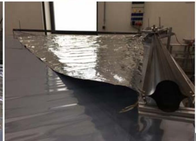
ADEO demonstrator deployment, functionality test 1
