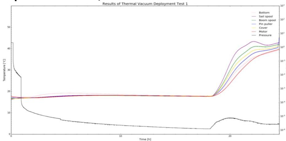
Temperature and vacuum profile before, after and during test
