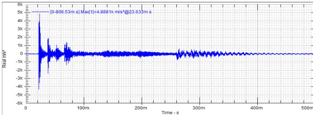
Acceleration measurement at HDRM activation
