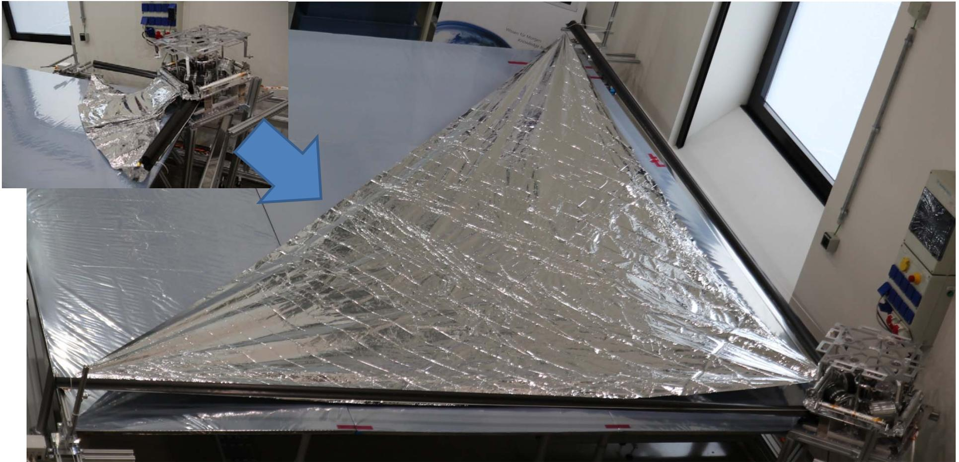
Full deployment successful: Demonstrator Test Campaign successful, raising TRL of ADEO to 5/6.
