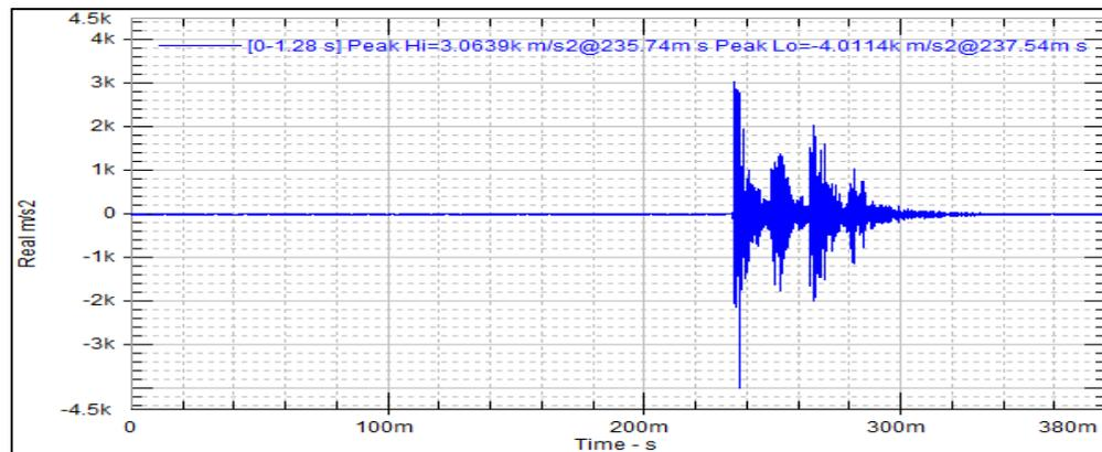
Acceleration measurement at HDRM activation
