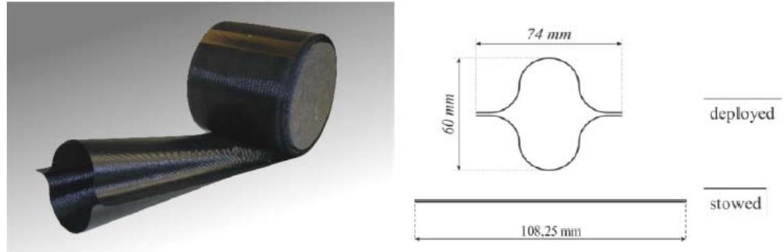
*Stowed CFRP boom deployed from coil*
