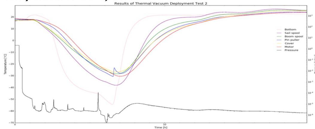
Temperature and vacuum profile before, after and during test
