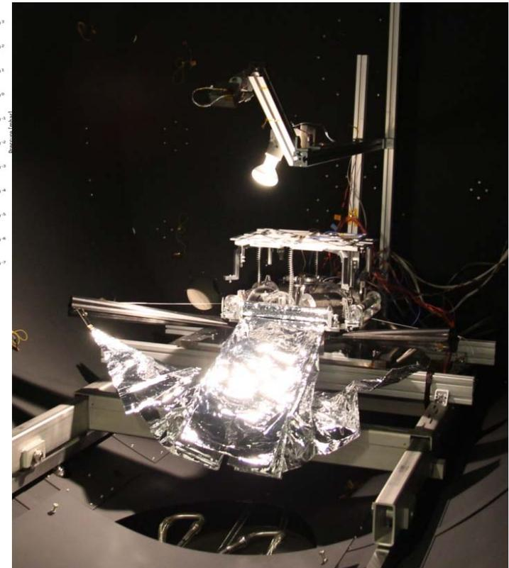
ADEO demonstrator partially deployed in TVAC chamber
