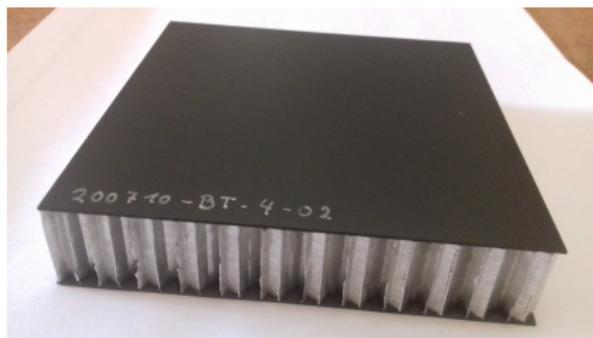
20mm aluminum honeycomb, CFRP facesheets as above
