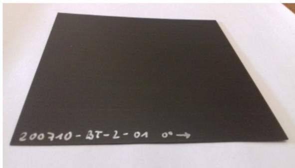
INVENT material, CFRP M55J fibres with EX1515 cyanate ester resin
