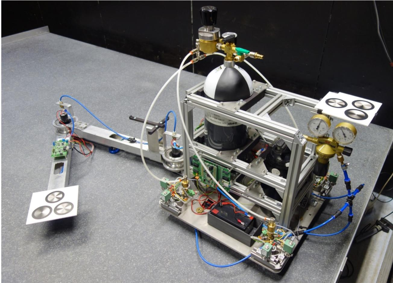
*Picture of the chaser satellite mock-up with attached 2 DoF manipulator.*
