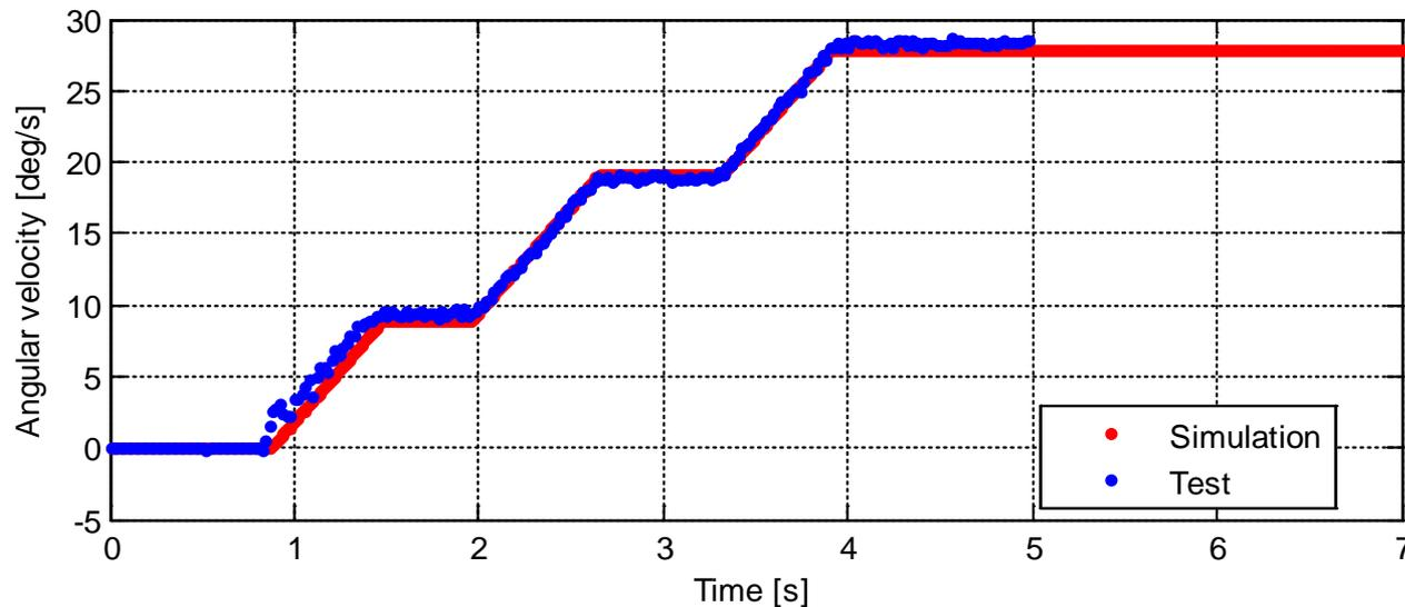
*Results of the thrusters performance test: linear and angular velocity.*
