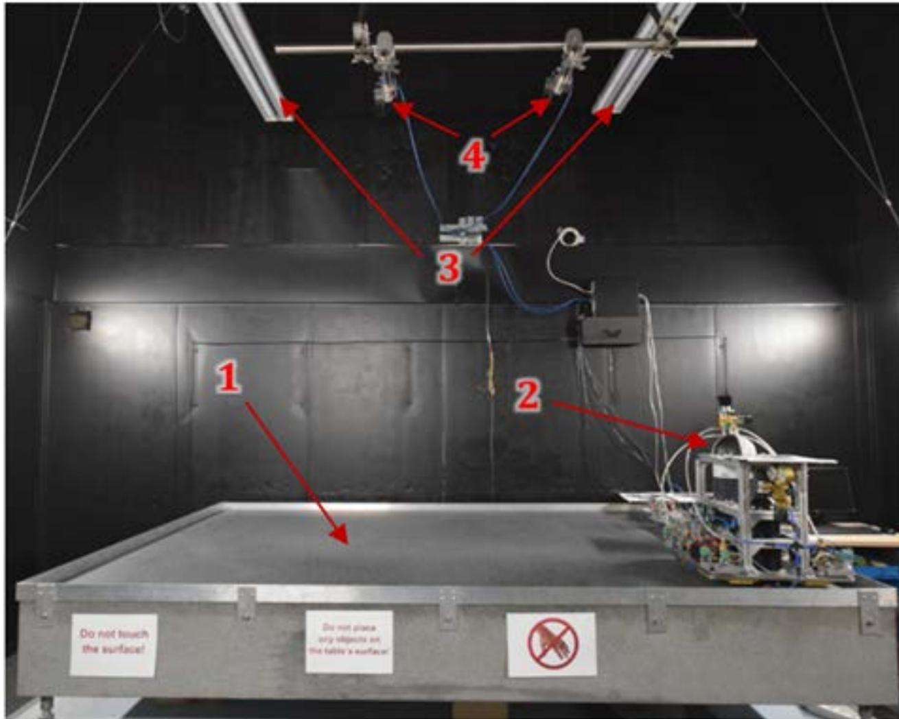
*Testing facility: 1 – air-bearing table, 2 – space robot, 3 – illumination system, 4 – vision system cameras.*
