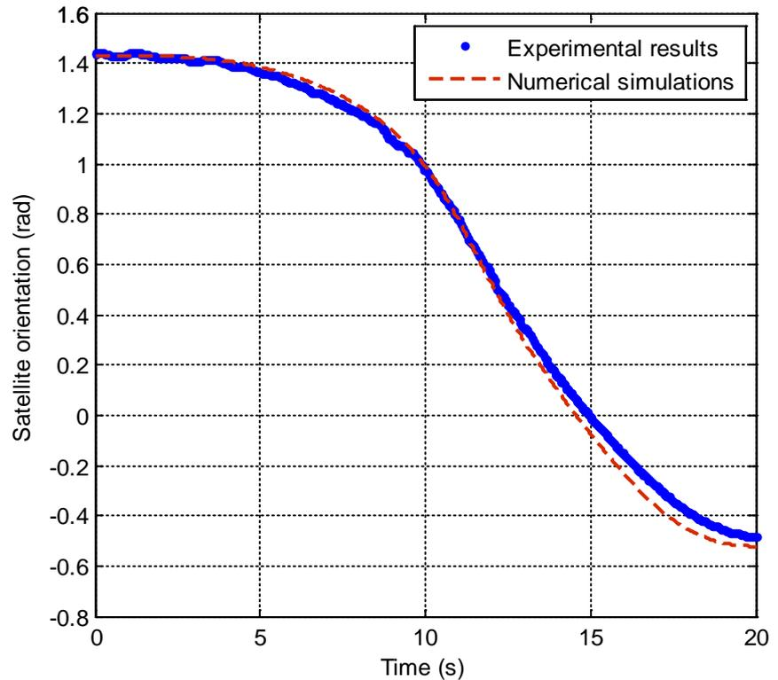
*Comparison between the satellite orientation obtained from numerical simulations and orientation of manipulator base measured during the experiment.*
