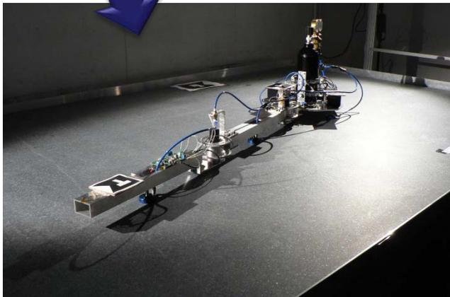
*Orbital capture manoeuvre with a manipulator (artist concept) and planar air-bearing microgravity simulator at CBK.*
