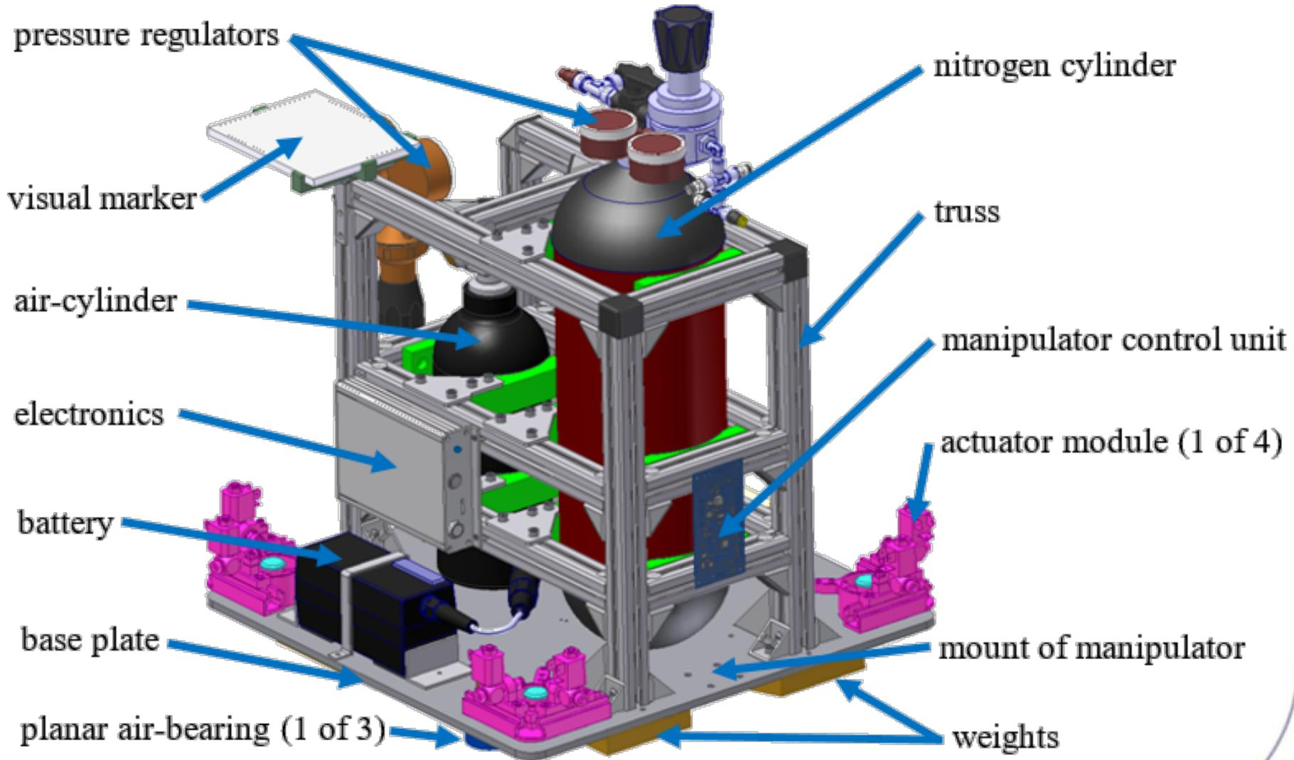
*The schematic view of the chaser satellite mock-up.*
