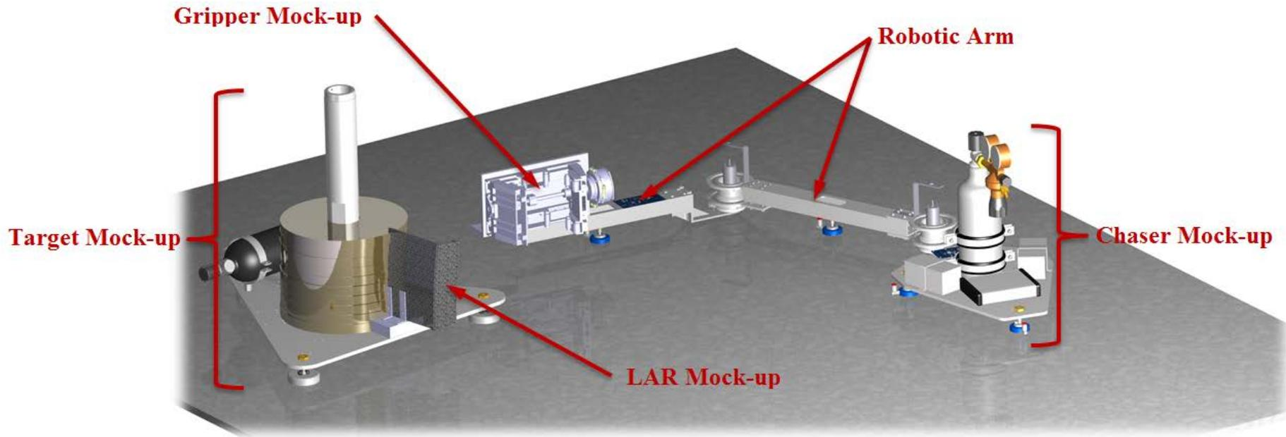
*Experimental test set-up on the planar air-bearing microgravity simulator with chaser and target mock-ups.*
