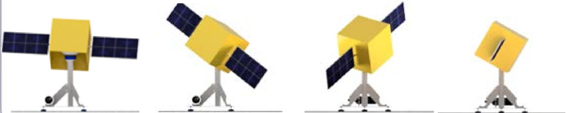
*The different positions of satellite mock-up achieved by using the spherical air-bearing.*
