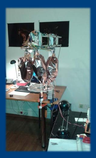
Pre-prototype built for concept verification and control loop tuning
