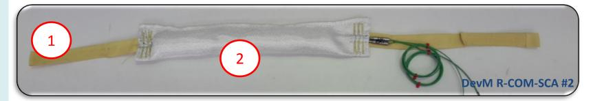
For the **Stiff Part** several high-strength and low flexibility fibers available in the market and with a known space heritage have been evaluated. At the end a **Kevlar** webbing 25 mm wide capable of withstanding 7750 N has been selected For the **Thermal Part** several materials have been evaluated (metals, ceramics and ablative). At the end the designed protection system is:
