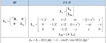
Compute the robot control output
