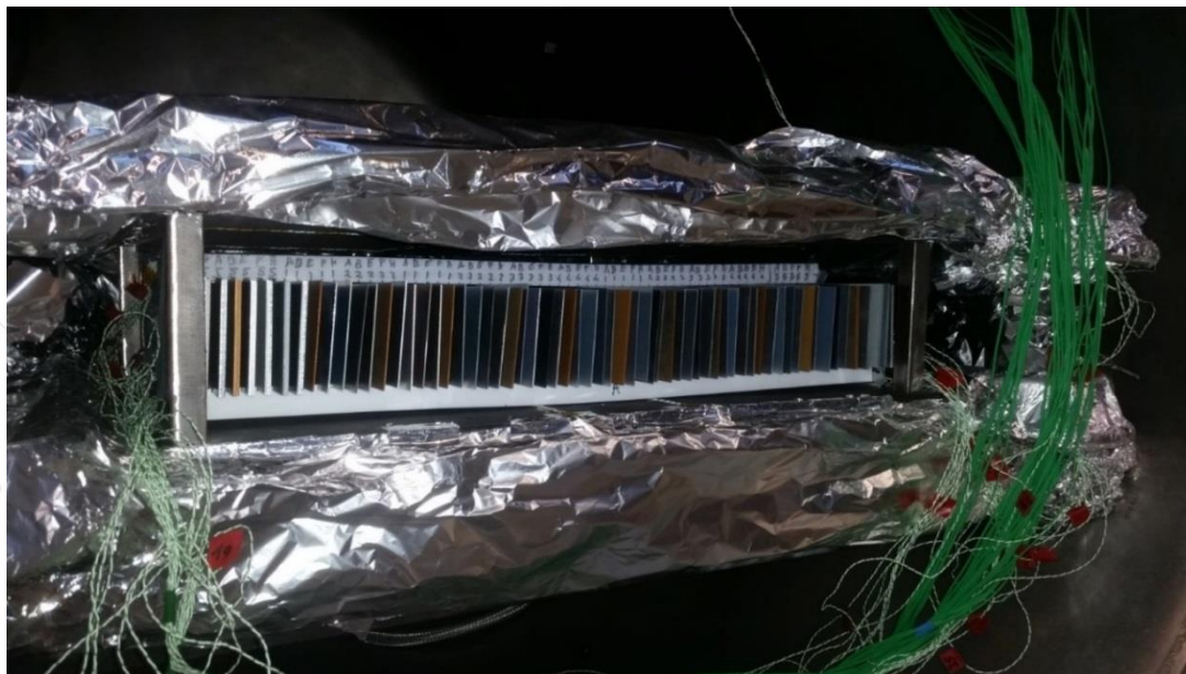
Figure 9 – Details of the test panels submitted to Thermal Cycling.
