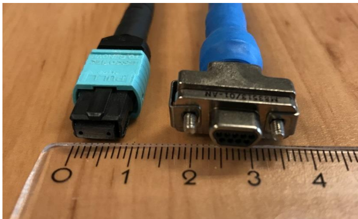
Optical connector with 6 SpFi links @ 10Gbps each smaller than single SpW connector at 200Mbps
