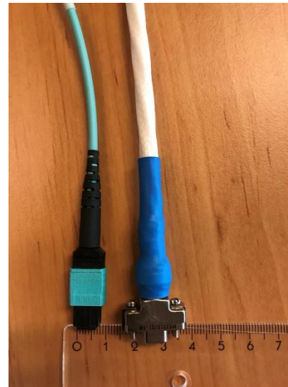
12 Fibre vs single SpW cable
