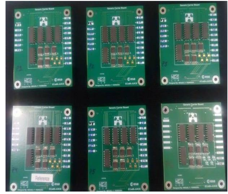
Transistor (Bipolar) 2N2222 OPAMP Analog ICs non ELDRS LM124 Voltage Reference Analog ICs displaying ELDRSLM4050
