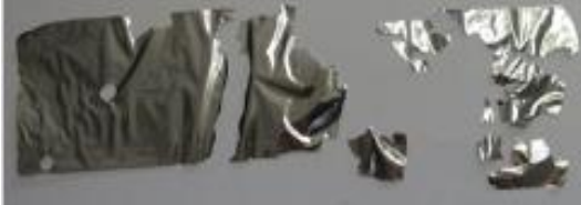
Debris of MLI internal layers
