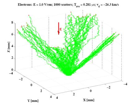
**Above:** e- (green) propagating in different conduction band minima. Image from Cabrera et al., 2010
